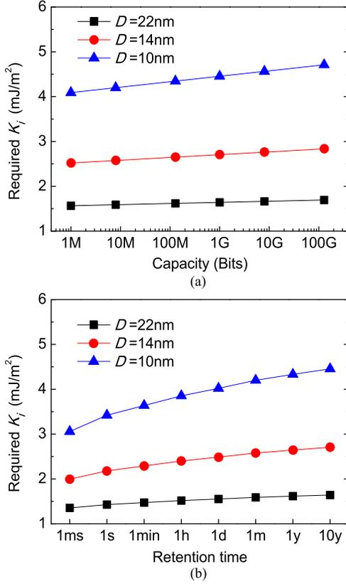
Fig. 4. Required interfacial anisotropy  $K_i$  as a function of (a) capacity and (b) retention time with different MTJ diameter  $D$ . (a) Retention time of 10 years is assumed. (b) Capacity of 1 Gbit is assumed.
