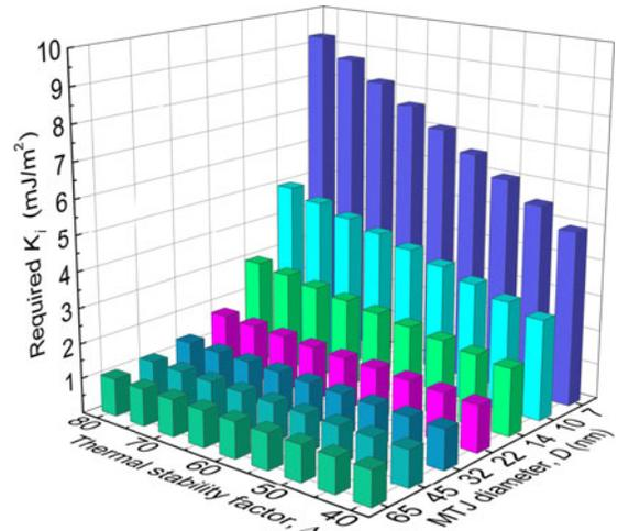
Fig. 3. Required interfacial anisotropy  $K_i$  as a function of thermal stability factor  $\Delta$  and MTJ diameter  $D$ .
