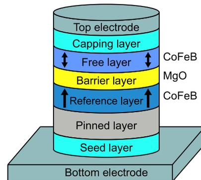
Fig. 1. Illustration of the MTJ stack based on the interfacial PMA of CoFeB/MgO/CoFeB structure.
