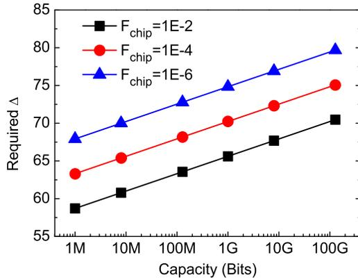
Fig. 2. Dependence of required thermal stability factor  $\Delta$  on capacity with different chip failure rates  $F_{\text{chip}}$ . The points correspond to capacities of 1 Mbit, 8 Mbit, 128 Mbit, 1 Gbit, 8 Gbit, and 128 Gbit.
