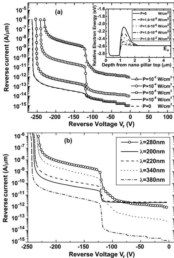
Fig. 4. (a) Simulated  $I$ - $V$  characteristics of 4H-SiC NAPD under illumination with different power densities at  $\lambda = 280$  nm and (b) with different wavelengths under  $1.0 \times 10^{-2}$  W/cm<sup>2</sup> illumination. The avalanche voltage and band diagram of NAPD are dependent on power density and wavelength of the incident illumination.
