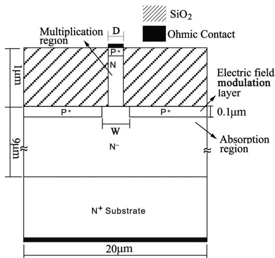
Fig. 1. Structure of 4H-SiC nano-pillar APD.
