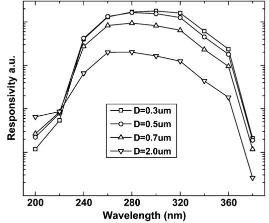
Fig. 3. Simulated spectral responsivities of 4H-SiC NAPD with different pillar diameter ( $D$ ), under  $1.0 \times 10^{-2} \text{ W/cm}^2$  illumination. The bias of NAPD is the  $95\% \times V_{\text{br}}$  of the NAPD under  $1.0 \times 10^{-2} \text{ W/cm}^2$  illumination with wavelength of 280 nm.
