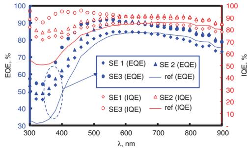
**Fig. 2** Results of external and internal quantum efficiencies (EQE, left; IQE, right) measurements by three different processes on large-size mc-Si solar cells; corresponding data of reference cell also plotted as comparison
