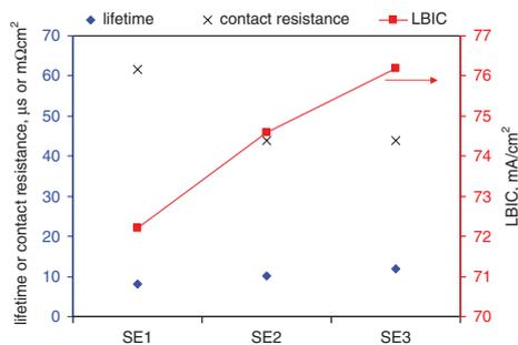
**Fig. 3** Comparison with lifetime (in  $\mu\text{s}$ ), contact resistance (in  $\text{m}\Omega/\text{cm}^2$  both at left axis) and LBIC (in  $\text{mA}/\text{cm}^2$  at right axis) on mc-Si solar cells developed by three different SE processes
