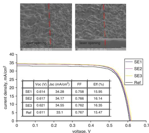
**Fig. 1** Current density-voltage ( $J\text{--}V$ ) characteristics of selective emitter (SE) multi-crystalline silicon (mc-Si) solar cells with different process schemes
