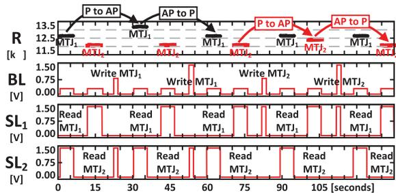
Fig. 4. Measured transient waveforms for reading and writing the crossbar array, demonstrating that  $MTJ_1$  can be written with unipolar set/reset voltages (0.5 and 1.1 V, respectively) and read without disturbing  $MTJ_2$  and vice versa. A sensing voltage of 0.2 V in the SL is used for the read process, while unaccessed SLs are pulled to  $V_{DD}$  (1.5 V).
