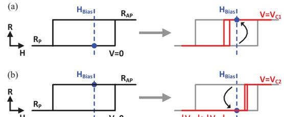
Fig. 1. Writing of the VCMA-based MTJs in the  $P$  to  $AP$  direction is accomplished by a voltage  $V_{C1}$ , which reduces the coercivity of the free layer and results in a single available state at the bias field  $H_{Bias}$  provided by the fixed layer. Further increasing the magnitude of the voltage to  $V_{C2}$  allows STT to switch the device in the opposite (e.g.,  $AP$  to  $P$ ) direction [6], [7].
