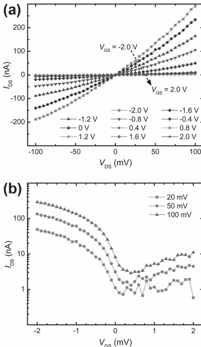
**Figure 3.** The experimental *I*–*V* characteristics of the MoO<sub>3</sub> FET. (a) *I*<sub>DS</sub> vs. *V*<sub>DS</sub> characteristics of the FET with varying back-gate voltages (*V*<sub>GS</sub>) in steps of 0.4 V from -2 to +2 V. (b) Corresponding *I*<sub>DS</sub>–*V*<sub>GS</sub> curves of the FET acquired at *V*<sub>DS</sub> values of 20, 50, and 100 mV.
