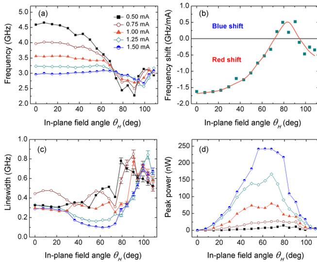
FIG. 3. (Color online) (a) Frequency, (b) frequency shift, (c) linewidth, and (d) integrated power of the first peak as a function of in-plane field angle  $\theta_H$ . The solid curve in (c) is added as a guide for the viewer.
