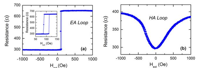
FIG. 1. (Color online) Resistance as a function of in-plane field  $H_{ext}$  for the same device for fields (a) along the easy-axis direction and (b) along the hard-axis direction. Inset in (a) is the magnified view in the low-field range.
