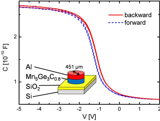
**Figure 2.**  $C$ - $V$  characteristics obtained from two circular MOS capacitors with radius  $r = 451 \mu\text{m}$  as shown in the inset. Both the forward (from negative to positive voltages) and the backward (from positive to negative voltages) sweep are shown for each sample. We obtain  $\Phi_M = 4.237 \text{ V}$  as the work function of  $\text{Mn}_5\text{Ge}_3\text{C}_{0.8}$  from the measurements.
