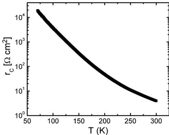
**Figure 4.** Temperature dependence of the specific contact resistivity as measured between adjacent contact pads of a TLM structure of sample B for temperatures between 70 and 300 K. The specific contact resistivity shows a strong temperature dependence as temperature is decreased.
