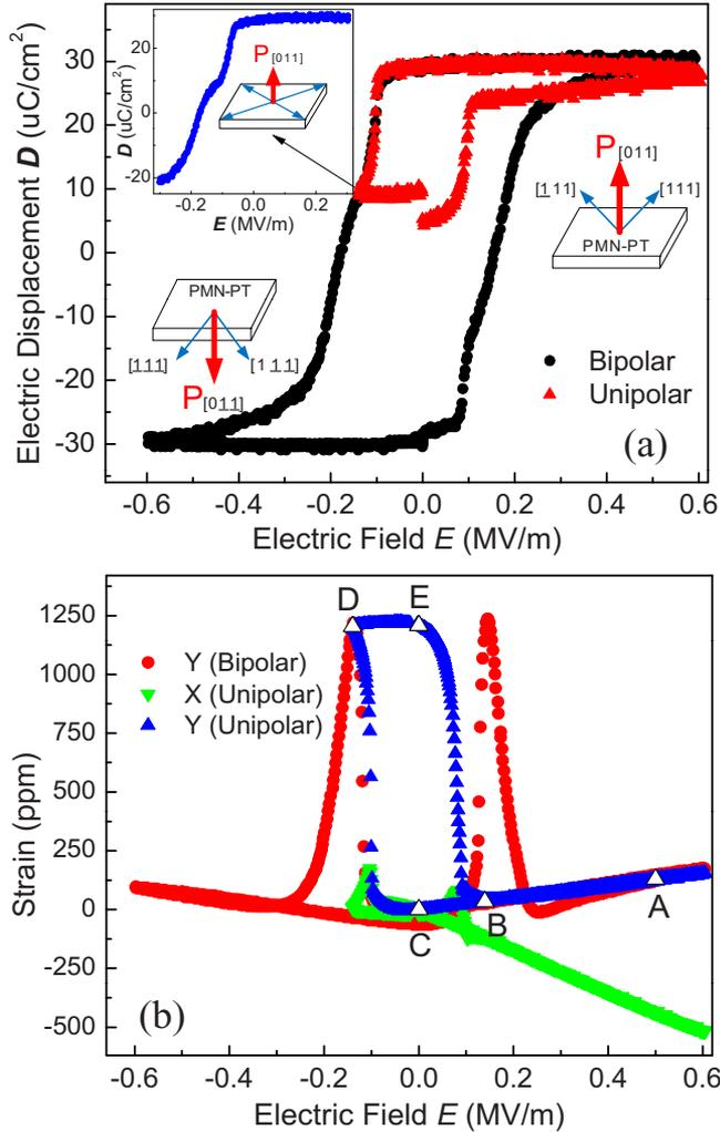
FIG. 2. (Color online) (a) Out-of-plane ( $\bar{z}$  direction) electric displacement as a function of electric field. (b) In-plane piezoelectric strain value along the  $\bar{x}$  and  $\bar{y}$  directions.
