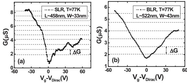
FIG. 3. Four-probe transport properties of SLR and BLR at  $T=77$  K. (a)  $G$ - $V_g$  curves of a SLR ( $L\sim 458$  nm,  $W\sim 33$  nm). (b)  $G$ - $V_g$  curves of a BLR ( $L\sim 522$  nm,  $W\sim 43$  nm). The conductance quantization was observed at 77 K for both SLR and BLR. Horizontal dashed lines are guides for eyes, showing the quantization spacing of the conductance  $\Delta G_{\text{SLR}}\sim 0.7$   $\mu\text{S}$  and  $\Delta G_{\text{BLR}}\sim 0.6$   $\mu\text{S}$ , respectively.
