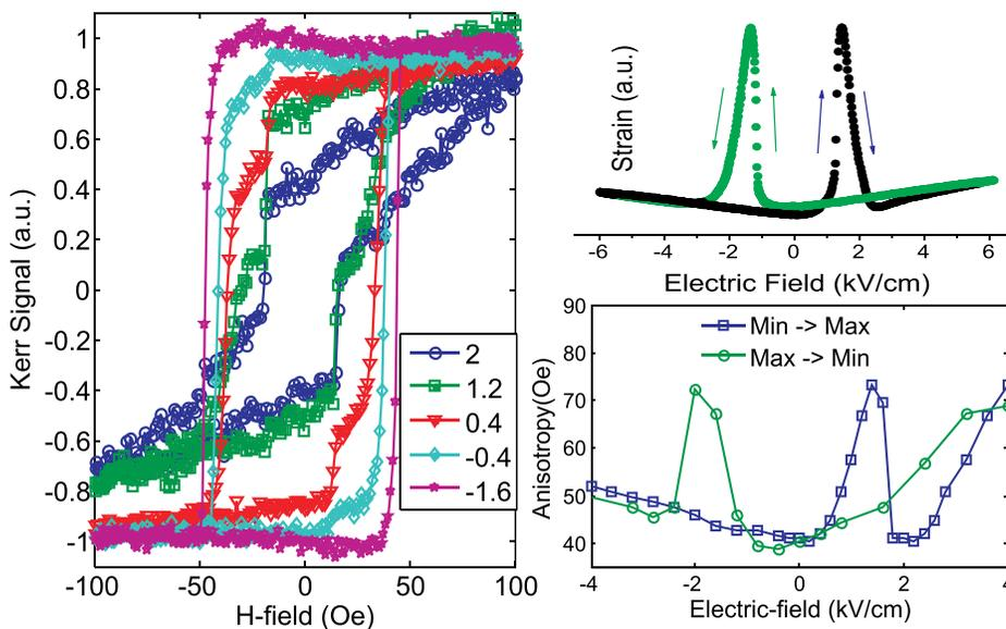
FIG. 2. Left: Kerr hysteresis curves at different electric fields given in units of kV/cm. Upper right: Strain response of PMN-PT as a function of electric field. The arrows indicate the electric field sweeping direction. Lower right: Anisotropy field derived from the MOKE hysteresis curves as a function of electric field.
