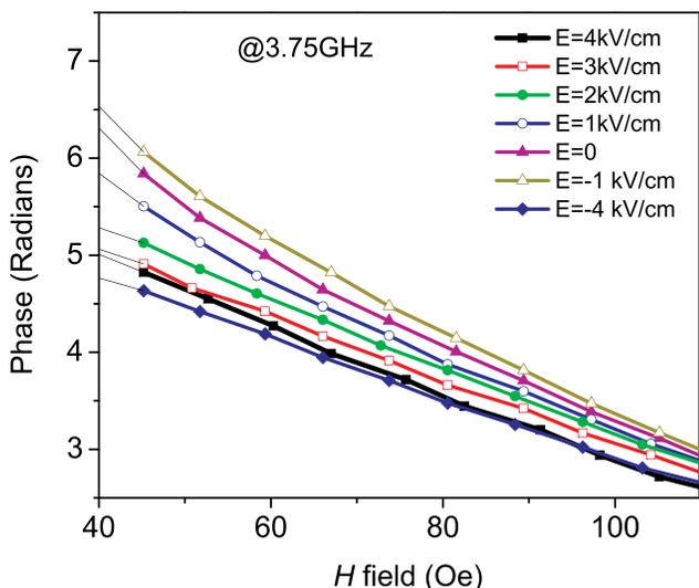
FIG. 4. Measured phase shift of the spinwaves at different electric fields for one fixed frequency.
