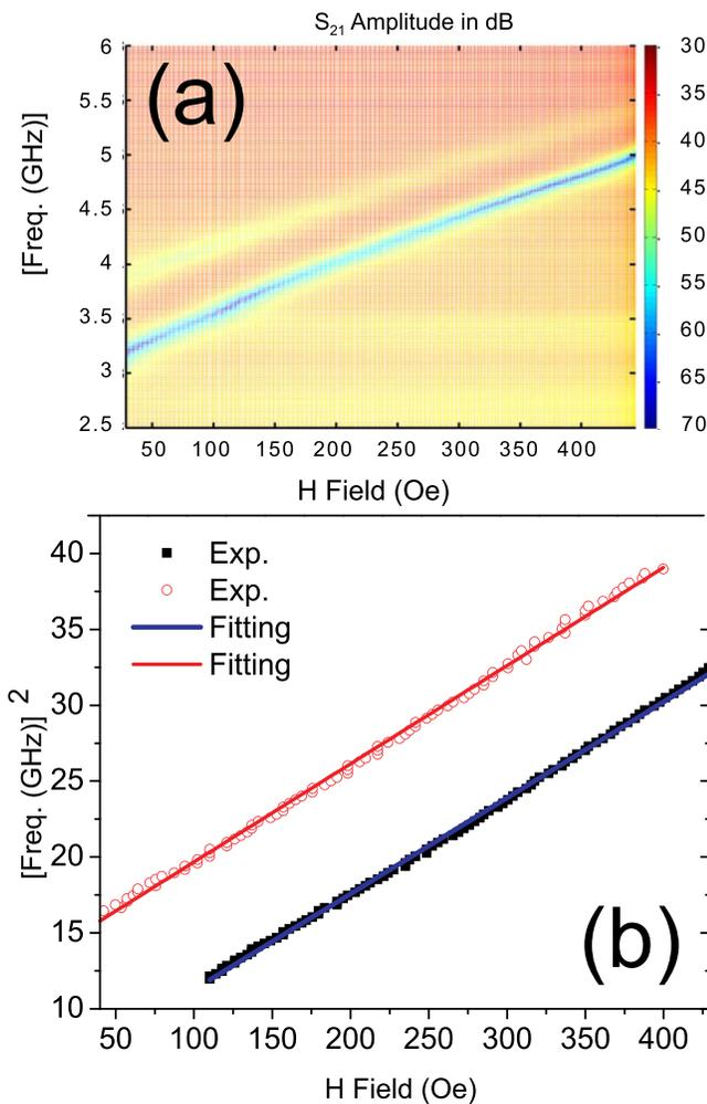
FIG. 3. Top:  $S_{21}$  response measured by network analyzer showing the distinct spinwave features. Bottom: Fitting of the experimental data to the Damon and Eschbach surface mode spinwaves.
