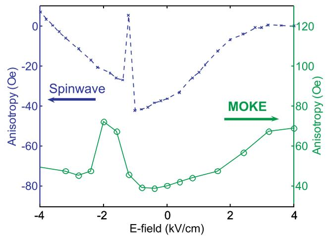
FIG. 5. Left axis: Effective anisotropy field vs electric field derived from spinwave data. Right axis: Effective anisotropy field derived from Kerr hysteresis loops (Fig. 2).
