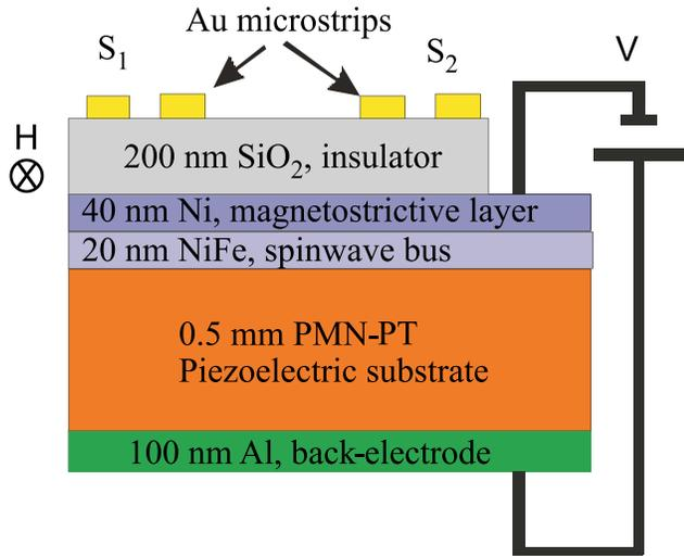
FIG. 1. Cross section of device layer structure and experimental configuration of spinwave excitation ( $S_1$ )/detection ( $S_2$ ) antennas, bias magnetic field, and bias electric field.
