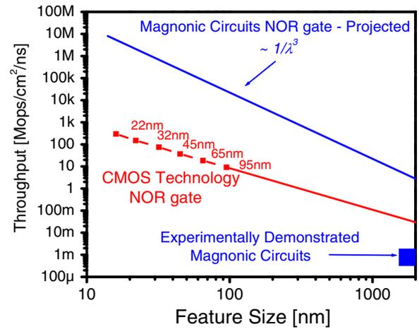
**Figure 4.** Numerical estimates on the functional throughput of the Magnonic majority logic gate (can be used as AND or OR gates) and conventional CMOS-based NOR gate. The throughput is plotted as a function of the minimum feature size, which is the gate length for CMOS and the wavelength  $\lambda$  for spin wave circuit, respectively. (This figure is in colour only in the electronic version)
