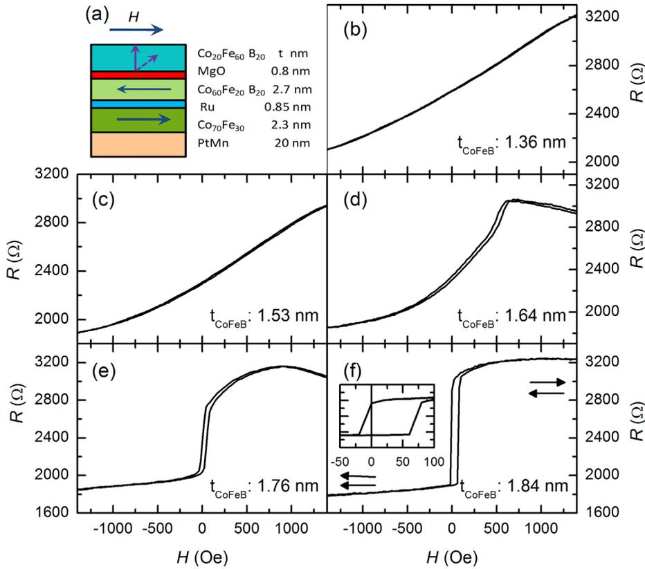
FIG. 1. (a) Layer structure and magnetic configuration of sensors. (b)-(f) Resistance as a function of the applied magnetic field for the sensors with different thickness ( $t_{\text{CoFeB}}$ ) of the sensing CoFeB layer. The inset in (f) shows the minor loop.
