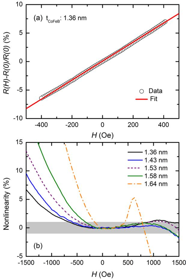
FIG. 2. (a) Resistance as a function of applied magnetic field curve for a sensor with CoFeB sensing layer of  $t_{\text{CoFeB}} = 1.36$  nm in the low magnetic field regime. (b) Nonlinearity in the magnetoresistance for different CoFeB sensing layer thickness. The light gray box in (b) illustrates the range where nonlinearity is less than 1%.
