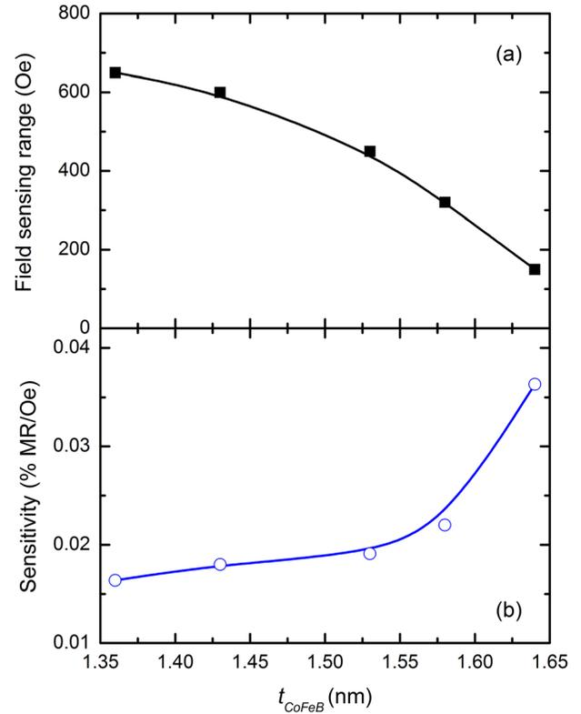
FIG. 3. Field sensing range (a) and sensitivity (b) as a function of the CoFeB sensing layer thickness. The data are deduced from Fig. 2(b) when the nonlinearity is less than 1%. Note that the values corresponding to nonlinearity of 1% for negative fields are smaller than those for positive fields; thus, the negative data are used in this letter. The line in (a) and (b) is a guide for the eye.
