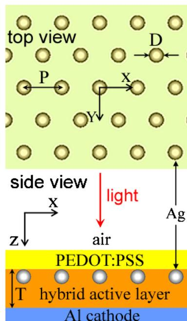
FIG. 1. (Color online) Schematic structure of the simulated plasmonic OPV cell. The symbols, T, D, and P, are active layer thickness, nanosphere diameter, and period, respectively.
