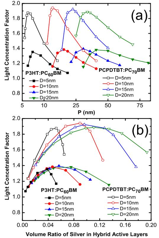
FIG. 3. (Color online) For  $D=5, 10, 15,$  and  $20$  nm and  $T=40$  nm in P3HT:PC<sub>60</sub>BM and PCPDTBT:PC<sub>70</sub>BM, (a) Light concentration factor as a function of nanosphere period  $P$ , (b) Light concentration factor as a function of volume ratio of silver in hybrid active layers.
