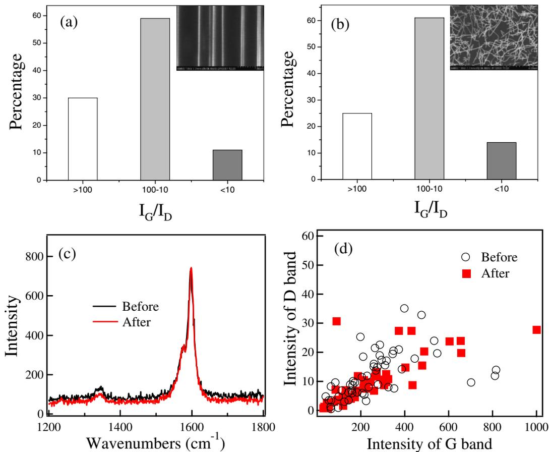
**Fig. 2.** (Color online) Defect analysis for aligned nanotubes on quartz (a) and randomly grown nanotubes on Si/SiO<sub>2</sub> (b). (c) Raman spectra of a nanotube before (black) and after (red) transfer, showing little difference. (d) Raman intensity of D- and G-bands of an ensemble of 60 nanotubes before and after transfer.
