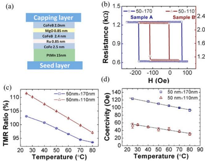
Fig. 1. (a) Schematic of an MTJ device stack structure. (b) Resistance versus magnetic field loop of Sample A (50 nm × 170 nm) and Sample B (50 nm × 110 nm). (c) and (d) TMR ratio and coercivity dependence on temperature of the two samples.
