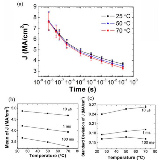
Fig. 4. (a) Current density from 10 ns to 0.1 s measured in Sample A. Each symbol represents the mean value and error bars indicate the standard deviation. (b) and (c) Mean and standard deviation of switching current density as a function of temperature measured in Sample A.
