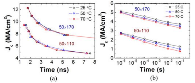
Fig. 2. (a) and (b) Switching current density at 50% switching probability versus pulse widths at short time scale (1–8 ns) and long time scale (1 μs–0.1 s).
