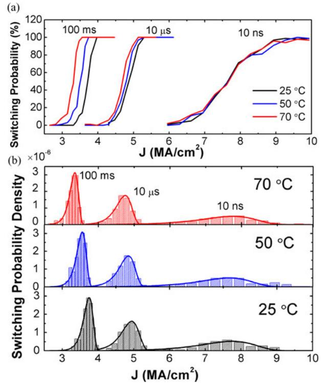
Fig. 3. (a) Switching probability as a function of current density measured in Sample A at 100 ms, 10  $\mu$ s, and 10 ns. (b) Switching probability density of sample A. The bars are experimental data and solid curves are fitted data.
