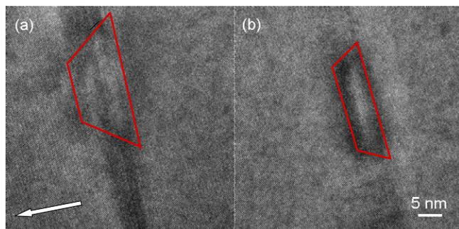
**Figure 3.** The HRTEM images recorded from an InAs quantum dot in layer 1 in (a) and layer 2 in (b). The arrow indicates the growth direction.
