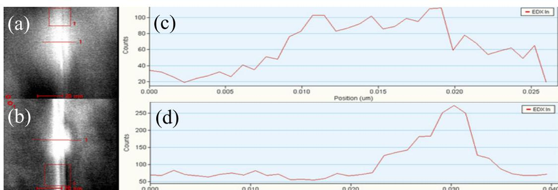
**Figure 4.** The STEM images recorded from the quantum dot in layer 1 in (a) and layer 2 in (b). The growth direction is horizontally leftwards for the two images. The corresponding EDX line profile of indium for the QD in layer 1 is shown in (c) and layer 2 in (d).
