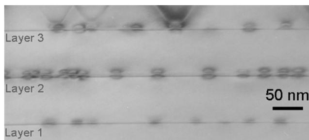
**Figure 2.** The bright field images recorded under  $g = 002$  of sample B showing the QD layers. The growth direction is vertically upwards for the images.
