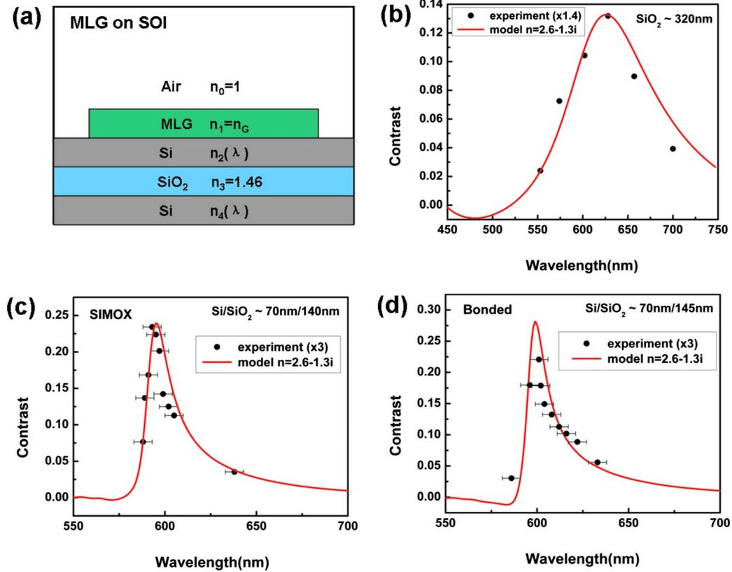
FIG. 2. (Color online) Contrast of graphene on SOI depending on wavelength. (a) Four-layer structure of MLG on SOI. (b) Contrast of MLG on  $\text{SiO}_2$ . (c) Contrast of MLG on SIMOX SOI. (d) Contrast of MLG on Bonded SOI. The error bars represent the FWHM=10 nm of the variable interference filter. The experimental values show good agreement with the simulation upon multiplying a constant as shown in each figure.
