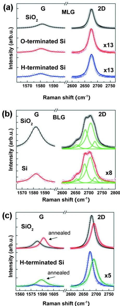
FIG. 3. (Color online) Raman spectroscopy (RS) of graphene on SOI. (a) RS of MLG depending on the polarity of Si surface. (b) RS of BLG on Si. The 2D band is fitted with four Lorentzian functions. (c) RS of graphene on SiO<sub>2</sub> are illustrated as reference. The Raman was taken at a condition of 600s acquisition time with less than 2 mW laser power. The Raman intensity for Si substrates are enhanced by a factor as indicated on each spectrum.
