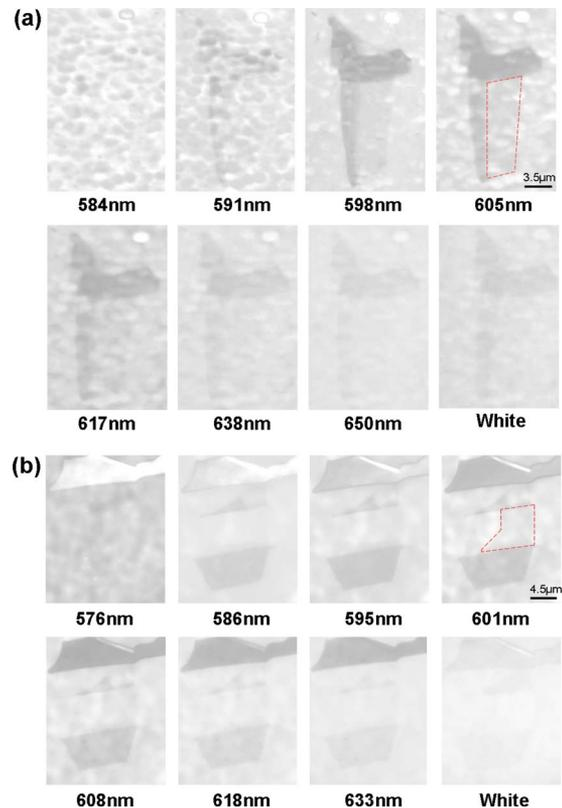
FIG. 1. (Color online) Optical images of graphene on SOI. (a) MLG on SIMOX SOI with different wavelengths of illumination. Scale bar: 3.5  $\mu\text{m}$ . (b) MLG on Bonded SOI. Scale bar: 4.5  $\mu\text{m}$ . The enclosed area of the dotted line is MLG. The images are illuminated through a narrow bandpass filter (variable interference filter).
