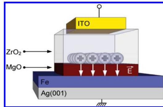
Fig. 9. Magnetoelectric charge-trap memory. An applied voltage pulse leads to the trapping of charges inside the dielectric layer of the device, which in turn exert an electric field on the  $\text{Fe}$ - $\text{MgO}$  interface, changing its anisotropy. The charge-trap memory state can thus be read out by measuring the magnetic state of the  $\text{Fe}$  layer. (Reprinted with permission from Ref. 65. Copyright 2012, American Chemical Society.)
