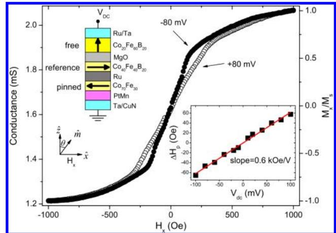
Fig. 2. Voltage-induced modulation of the perpendicular anisotropy in the free layer of a MTJ, observed by magnetoresistance measurements. The free layer is designed to have an out-of-plane magnetization, while the pinned layer is in-plane. The insets show the magnetic material stack and the dependence of the anisotropy on applied voltage. (Reprinted with permission from Ref. 46. Copyright 2012, American Physical Society.)
