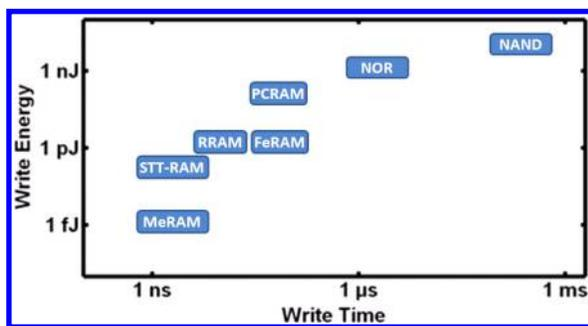
Fig. 10. Comparison of existing (NAND and NOR Flash) and emerging (MeRAM, STT-MRAM, Phase-Change, Ferroelectric and Resistive RAM) nonvolatile memory technologies in terms of energy dissipation and speed. MeRAM provides a significant improvement of energy efficiency, placing it in the preferred corner of the plot.
