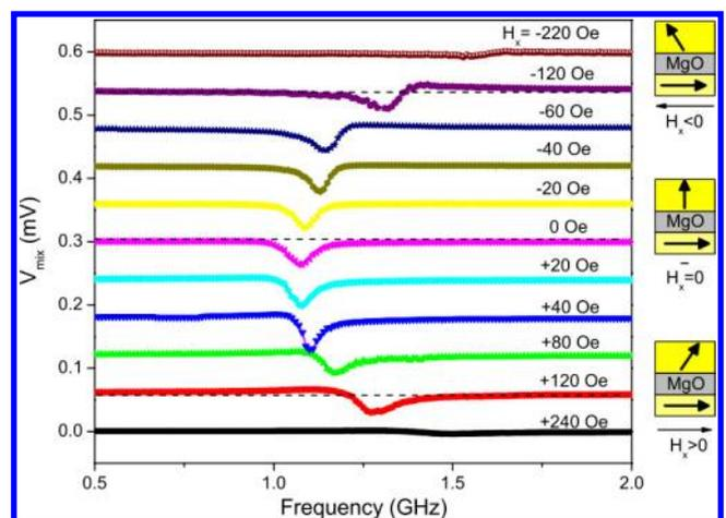
Fig. 4. VCMA-induced high-frequency magnetization dynamics in a MTJ. FMR spectra are obtained by measuring the rectified voltage across the junction when a RF signal is applied to it. Both STT and VCMA effects are present, and their relative contributions can be identified using the resonance line shape. (Reprinted with permission from Ref. 46. Copyright 2012, American Physical Society.)
