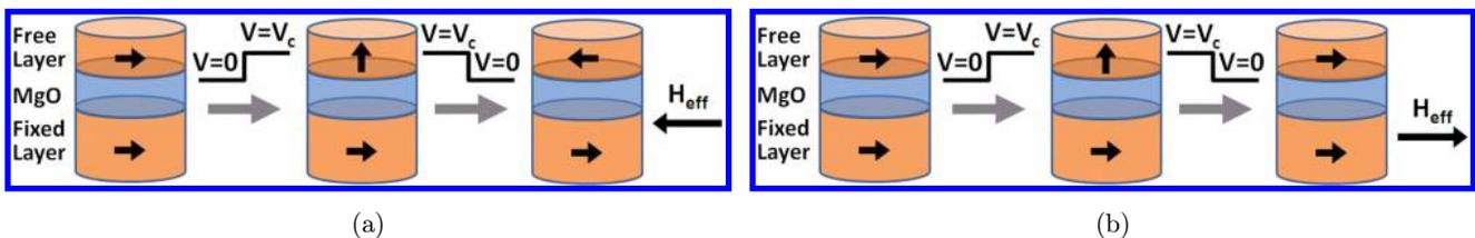
Fig. 6. Voltage-induced switching of an in-plane high-resistance MTJ. An applied voltage forces the magnetization into a metastable state, which then relaxes to a (similar or different) stable state after the voltage is removed.
