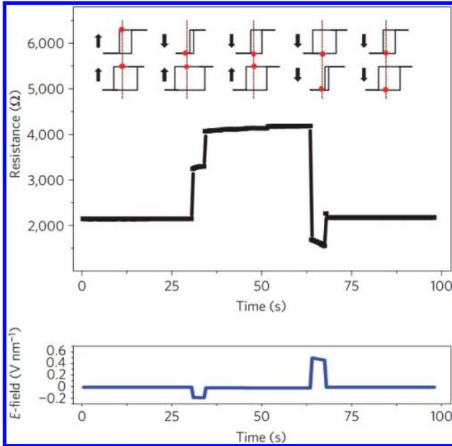
Fig. 7. Voltage-assisted switching of magnetization in a fully perpendicular MTJ. The switching is accomplished by modification of the free layer coercivity using an applied voltage, combined with the positioning of a DC bias magnetic field to accomplish switching. Top panel shows the measured resistance as a function of time, with the lower panel showing the applied electric field. (Reprinted with permission from Ref. 53. Copyright 2012, Macmillan Publishers Ltd: Nature Materials.)
